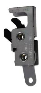
This Single Rotor Latch is a sub-platform to the TriMark proven 050-0500 series latch and is designed for light to medium-duty applications for on or off highway compartments and access panels. It features an extended trip mechanism for applications where it is desirable to have the release mechanism directly in-line with the latch.
